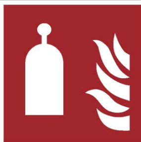
F014 Room protection alarm
