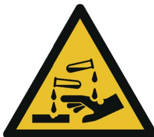
W023 Warning against caustic substances
