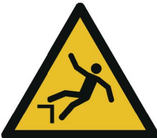
W008 Warning: Risk of falling
