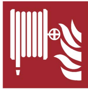
F002 Extinguishing hose
