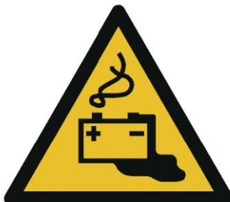
W026 Warning against danger caused by charging of batteries
