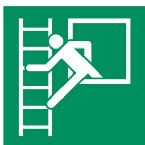
E016 Emergency exit with escape ladder
