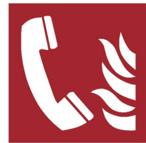
F006 Telephone for reporting fires
