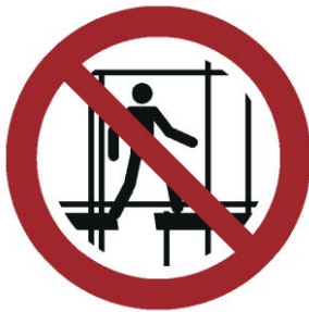
P025 Do not use the incomplete scaffold
