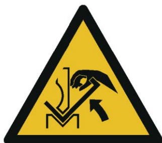
W031 Warning: Risk of squeezing the hand between the press and workpiece
